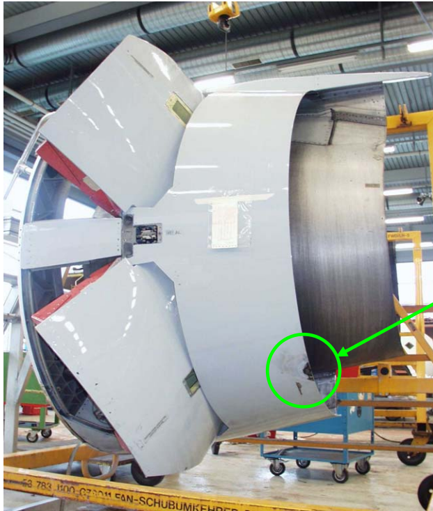
Lightning strike on CFM56-5A Fan Reverser
